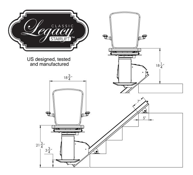
Model: SL14 Cap: 350 lbs Speed: 16 - 22 fpm Angle: 25 - 45 Power: 24vdc - 15a Drive: Rack & Pinion
