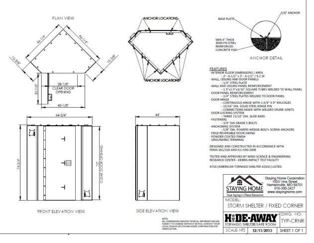
Position the **Corner Shelter upright.** Attach the roof / ceiling panel with nuts & bolts provided. Shim under the shelter walls as needed so the door swing clears.
