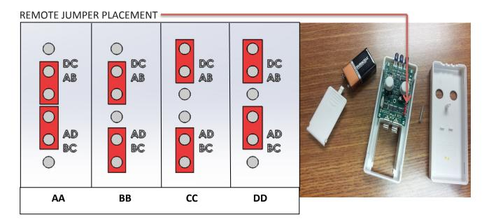
Change the corresponding code in the control board J1 jumper. The control board is located behind the panel on the downhill side of the chassis.
