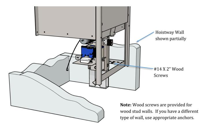
2. Attach (3) track brackets to each remaining piece of track.
